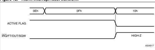
Figure 12. Alarm interrupt reset waveform
