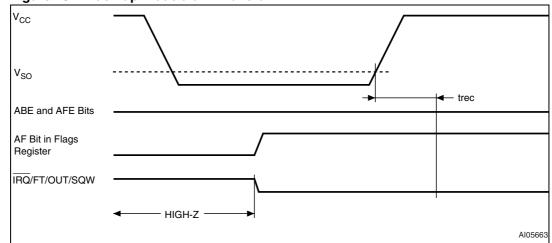
Figure 13. Back-up mode alarm waveform
