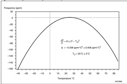
Figure 11. Clock calibration
