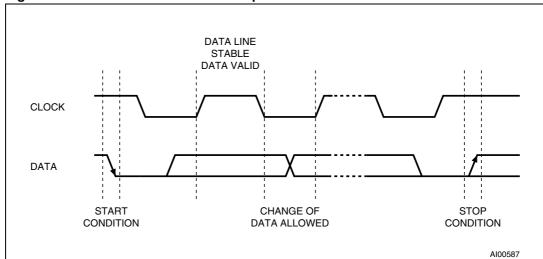
Figure 4. Serial bus data transfer sequence
