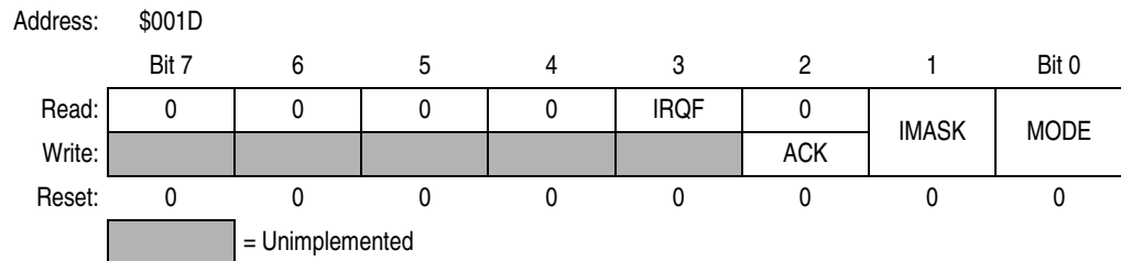
Figure 8-3. IRQ Status and Control Register (INTSCR)
