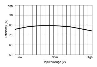
Efficiency vs Input Voltage
