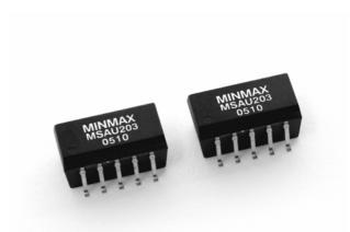
Minmax's MSAU200 1W DC/DC's are in "gull-wing" SMT package, weigh a mere 1.8 grams and meet 245°C/10sec in solder-reflow for lead free process.
