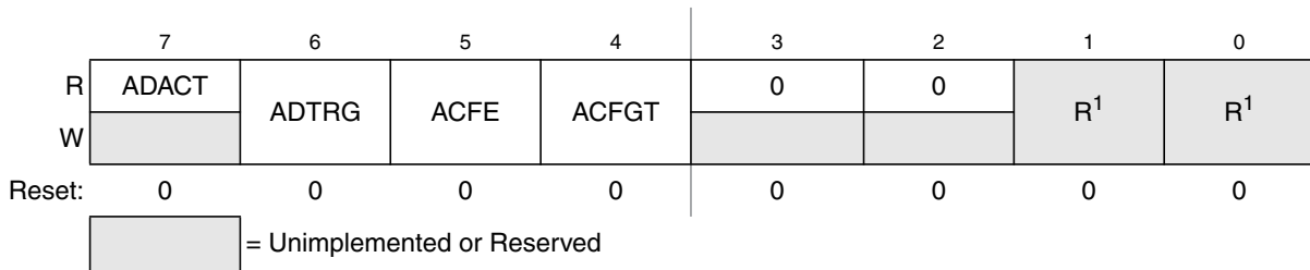
Figure 14-5. Status and Control Register 2 (ADC1SC2)
