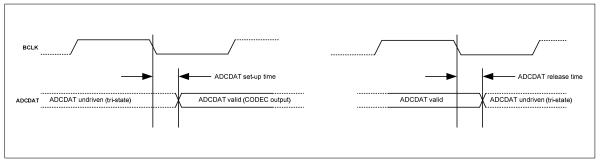
Figure 4 Audio Interface Timing – TDM Mode
