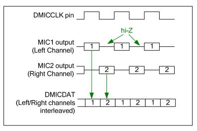
Figure 29 Digital Microphone Interface Timing
