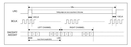
Figure 47 DSP Mode Audio Interface (mode B, AIF\_LRCLK\_INV=1, Slave)
