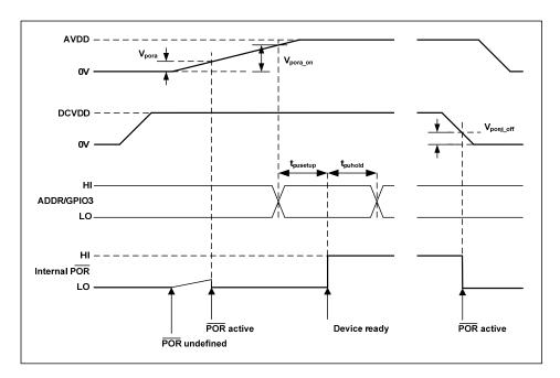
Figure 66 Power On Reset timing - DCVDD enabled first
