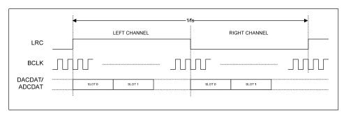
Figure 49 TDM in Left-Justified Mode
