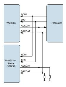
Figure 40 TDM with Processor as Master
