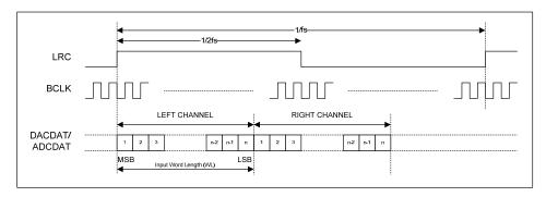
Figure 45 DSP Mode Audio Interface (mode B, AIF\_LRCLK\_INV=1, Master)
