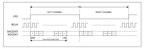
Figure 42 Left Justified Audio Interface (assuming n-bit word length)
