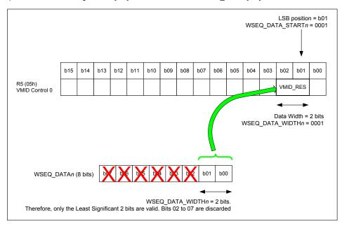
Figure 64 Control Write Sequencer Example
