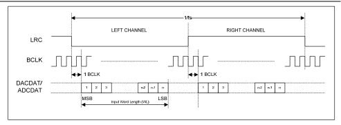
Figure 43 I2S Justified Audio Interface (assuming n-bit word length)
