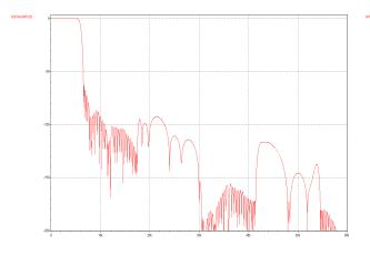
Figure 6 DAC Filter Response for CLK\_SYS\_MODE = 10b (Clock is 250 x fs related) DAC\_SB\_FILT = 1b (Sloping StopBand Filter) Sample Rate ≤ 24kHz
