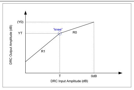
Figure 30 DRC Compression Characteristic
