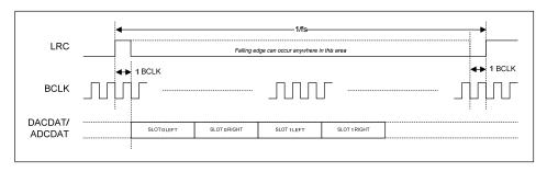
Figure 51 TDM in DSP Mode A
