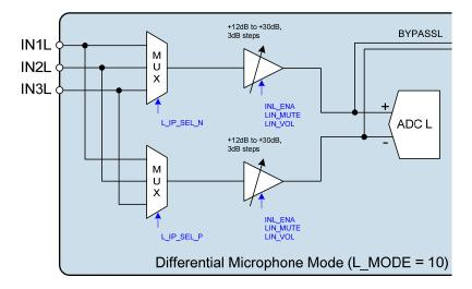
Figure 25 Differential Microphone Mode
