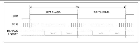
Figure 48 TDM in Right-Justified Mode
