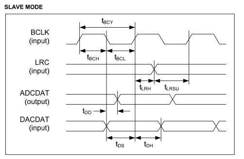
Figure 3 Audio Interface Timing – Slave Mode
