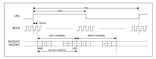
Figure 44 DSP Mode Audio Interface (mode A, AIF\_LRCLK\_INV=0, Master)
