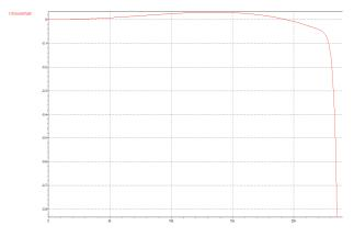
Figure 13 ADC Filter Passband Ripple for CLK\_SYS\_MODE = 10b
