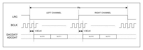
Figure 50 TDM in I<sup>2</sup>S Mode
