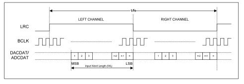
Figure 41 Right Justified Audio Interface (assuming n-bit word length)
