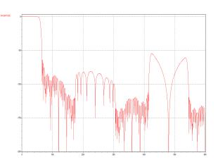
Figure 7 DAC Filter Response for CLK\_SYS\_MODE = 00b or 01b DAC\_SB\_FILT = 1b (Sloping StopBand Filter) Sample Rate ≤ 24kHz
