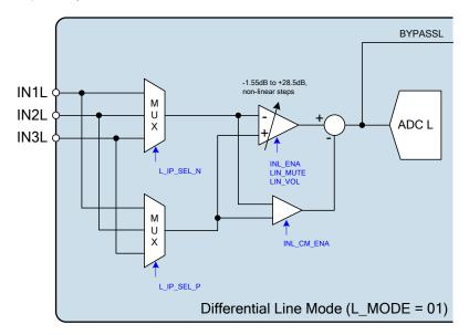
Figure 24 Differential Line Mode
