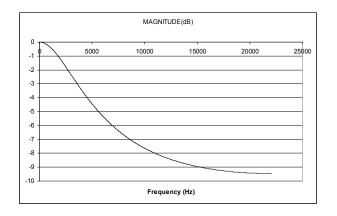
Figure 18 De-Emphasis Digital Filter Response (44.1kHz)
