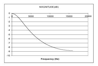
Figure 16 De-Emphasis Digital Filter Response (32kHz)
