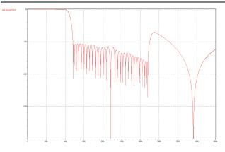
Figure 10 DAC Filter Response for CLK\_SYS\_MODE = 01b (Clock is 272 x fs related) DAC\_SB\_FILT = 0b (Normal Filter) Sample Rate = 88.2kHz
