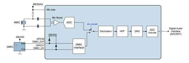
Figure 28 Digital Microphone Interface Control
