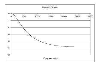
Figure 20 De-Emphasis Digital Filter Response (48kHz)
