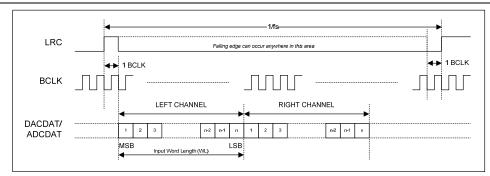
Figure 46 DSP Mode Audio Interface (mode A, AIF\_LRCLK\_INV=0, Slave)
