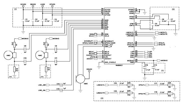
Figure 67 Recommended External Components
