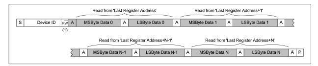
Figure 63 Multiple Register Read from Last Address using Auto-increment
