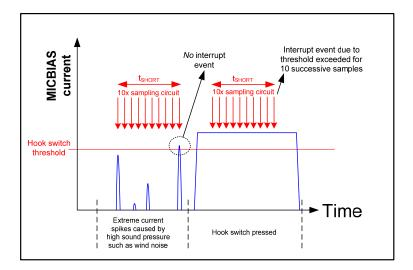
Figure 27 MICBIAS Hook Switch Detect Filtering
