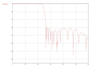
Figure 11 ADC Filter Response for CLK\_SYS\_MODE = 10b (not applicable to 88.2/96kHz)
