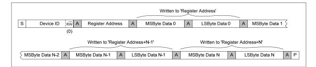
Figure 61 Multiple Register Write to Specified Address using Auto-increment
