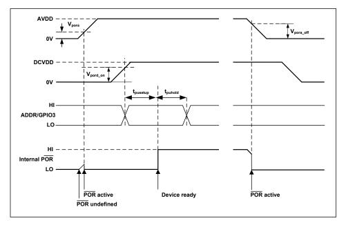
Figure 65 Power On Reset timing - AVDD enabled first
