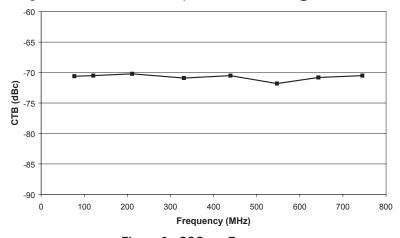
Figure 8: CSO vs. Frequency 112 Analog Channels, +34 dBmV Output Power, 3 dB Tilt @ 870 MHz, +8 V, 200 mA
