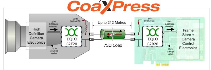
CoaXPress (CXP) is an asymmetric high speed point to point serial communication standard for the transmission of video and still images, scalable over single or multiple coaxial cables.
