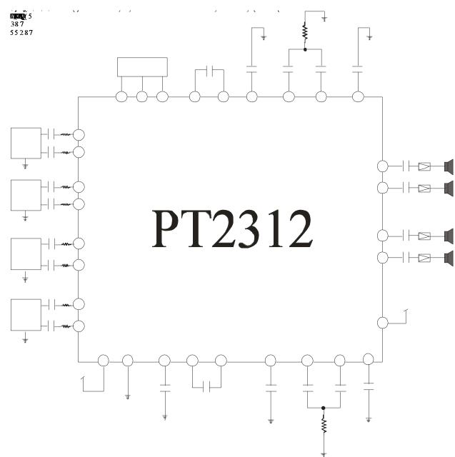
Notes: 1. The Resistor (R) Range = 2.0K Ohms to 3.6 K Ohms.
