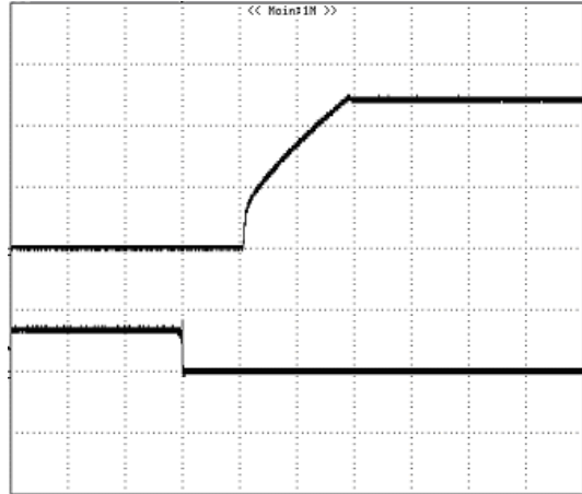
Figure 5: Turn-on transient at zero load current (5 ms/div). V_{in}=48V . Top Trace: V_{out} : 0.5V/div, Bottom Trace: ON/OFF input, 5V/div
