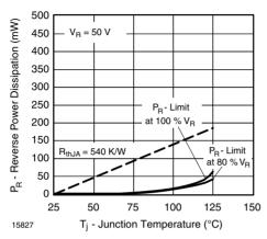
Figure 1. Max. Reverse Power Dissipation vs.
