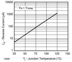
Figure 2. Reverse Current vs. Junction Temperature
