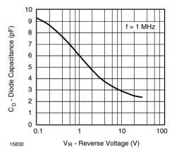
Figure 4. Diode Capacitance vs. Reverse Voltage
