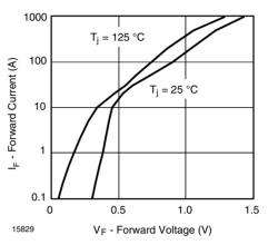
Figure 3. Forward Current vs. Forward Voltage
