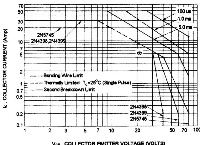
There are two limitation on the power handling ability of a transistor: average junction temperature and second breakdown safe operating area curves indicate  $I_c$ - $V_{ce}$  limits of the transistor that must be observed for reliable operation i.e., the transistor must not be subjected to greater dissipation than curves indicate.
