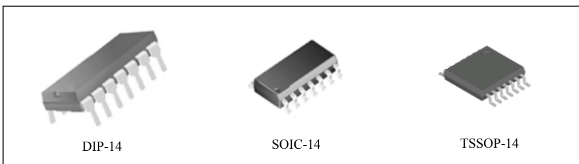
Figure 1. Package Types of AS324/324A
