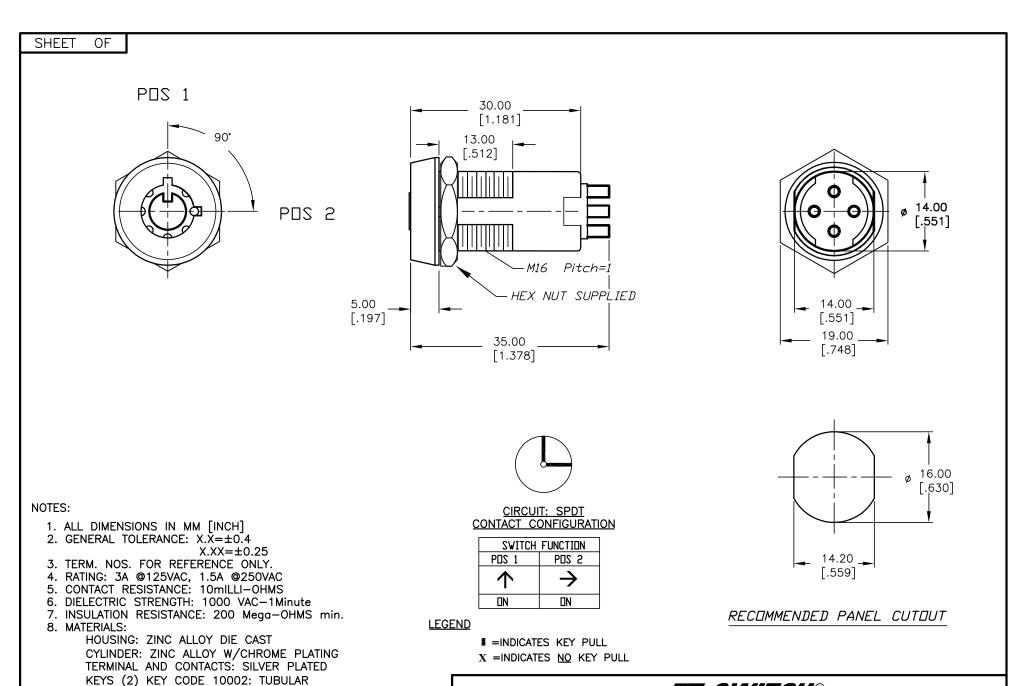
E-SWITCH® ZINC ALLOY, CHROME PLATING W/PLASTIC COVER TITLE К□104В-10007 13572 RELEASED FOR PRODUCTION Α 2/4/04 AR REV. ECN No. **DESCRIPTION** DATE CHKD SCALE DATE REV THE INFORMATION CONTAINED IN THIS DOCUMENT IS PROPRIETARY TO E-SWITCH AND IS NOT TO BE COPIED OR TRANSFERRED 2/4/04 AR K300108 1.5:1 Α
