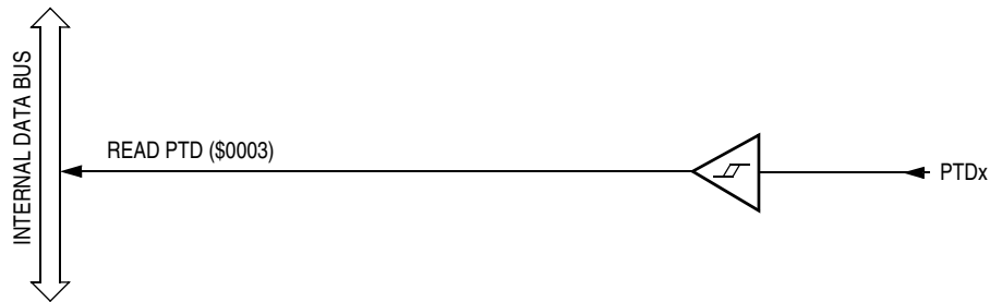
Figure 10-12. Port D Input Circuit
