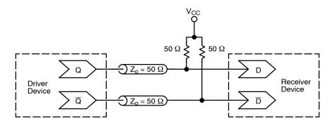
Figure 10. Typical Termination for Output Driver and Device Evaluation (See Application Note AND8057/D)
