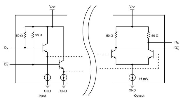
Figure 11. CML Input and Output Structure
