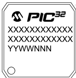
100-Lead TQFP (12x12x1 mm)
