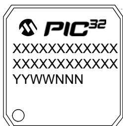
100-Lead TQFP (14x14x1 mm)
