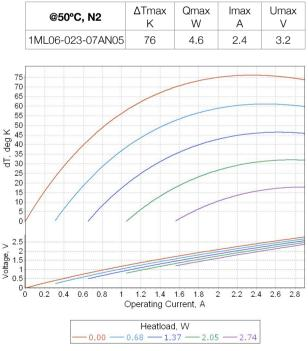
**Note**: Performance data is specified at optimal conditions (TEC hot side is stabilized at ambient temperature). Heatsink thermal resistance is not included into estimations. Use TECCad Software for estimations under different conditions.
