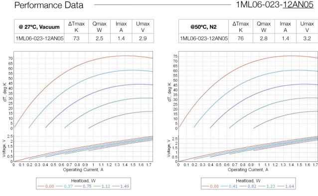
Note: Performance data is specified at optimal conditions (TEC hot side is stabilized at ambient temperature). Heatsink thermal resistance is not included into estimations. Use TECCad Software for estimations under different conditions.
