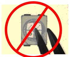
(2) In general, LEDs should only be handled from the side. By the way, this also applies to LEDs without a silicone sealant, since the surface can also become scratched.
