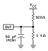
FIGURE 3. Output load circuit and test conditions
