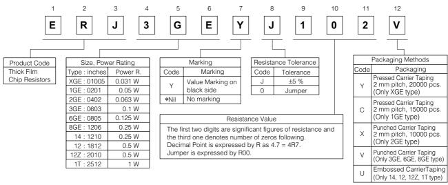
\* When omitted, the rest of the P/N factors shall be moved up respectively. (Only XGE, 1GE, 2GE type)
