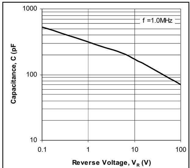
Figure 4. Typical Capacitance
