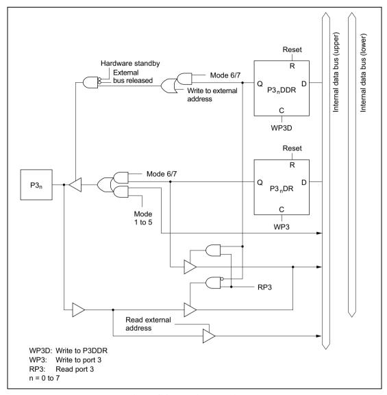
Figure C.3 Port 3 Block Diagram
