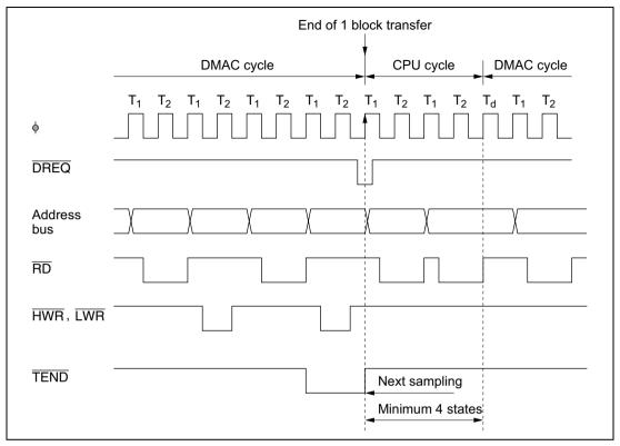
Figure 7.18 Timing of DMAC Activation by Falling Edge of DREQ in Block Transfer Mode
