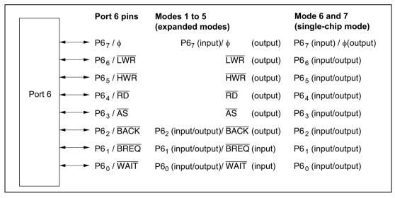
Figure 8.6 Port 6 Pin Configuration
