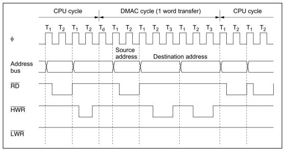
Figure 7.13 DMA Transfer Bus Timing (Example)
