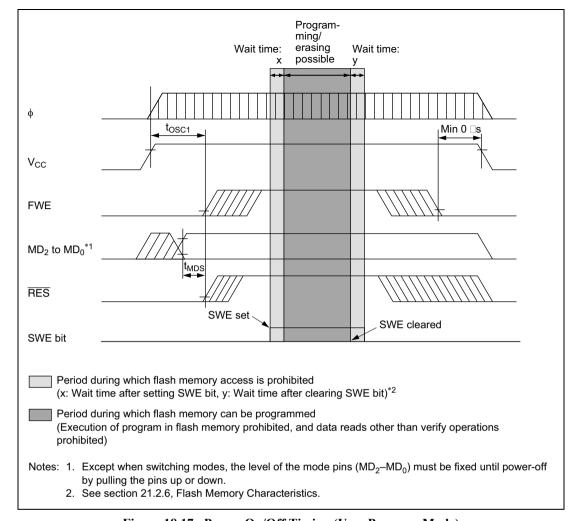
Figure 18.17 Power-On/Off Timing (User Program Mode)
