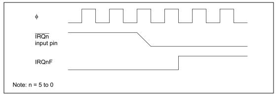
Figure 5.3 Timing of Setting of IRQnF
