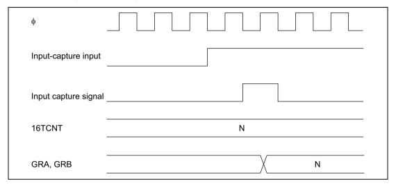
Figure 9.23 Input Capture Signal Timing
