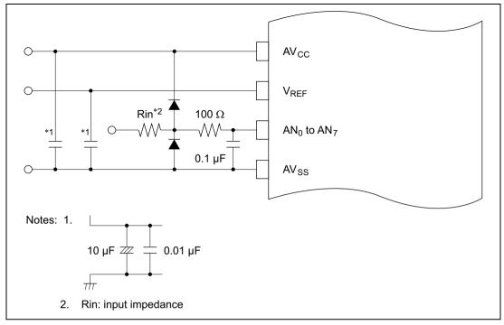
Figure 15.7 Example of Analog Input Protection Circuit
