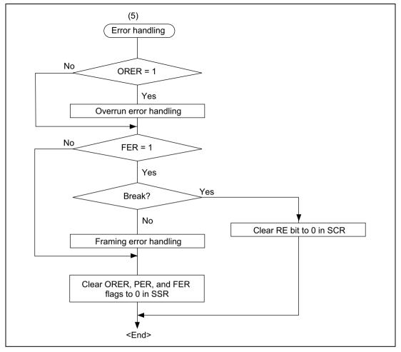
Figure 13.12 Sample Flowchart for Receiving Multiprocessor Serial Data (2)
