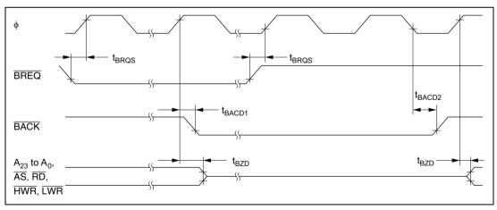
Figure 21.16 Bus-Release Mode Timing
