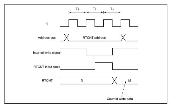
Figure 6.40 Contention between RTCNT Write and Increment
