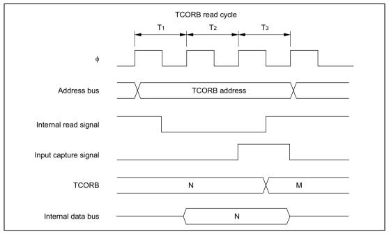
Figure 10.21 Contention between TCOR Read and Input Capture
