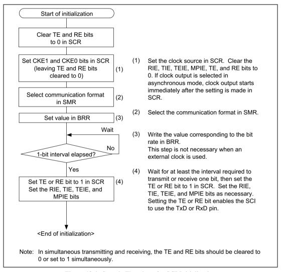
Figure 13.4 Sample Flowchart for SCI Initialization
