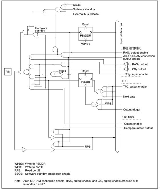
Figure C.11 (c) Port B Block Diagram (Pin PB<sub>2</sub>)
