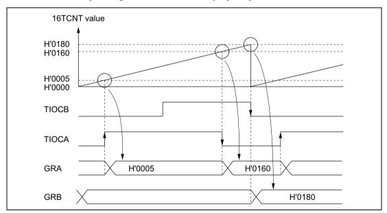
Figure 9.22 Input Capture (Example)
