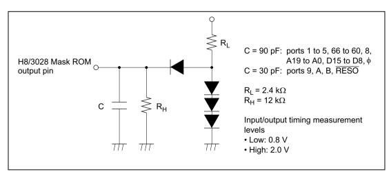
Figure 21.3 Output Load Circuit
