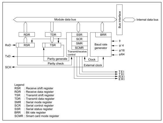
Figure 13.1 SCI Block Diagram
