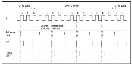
Figure 7.15 Burst DMA Bus Timing
