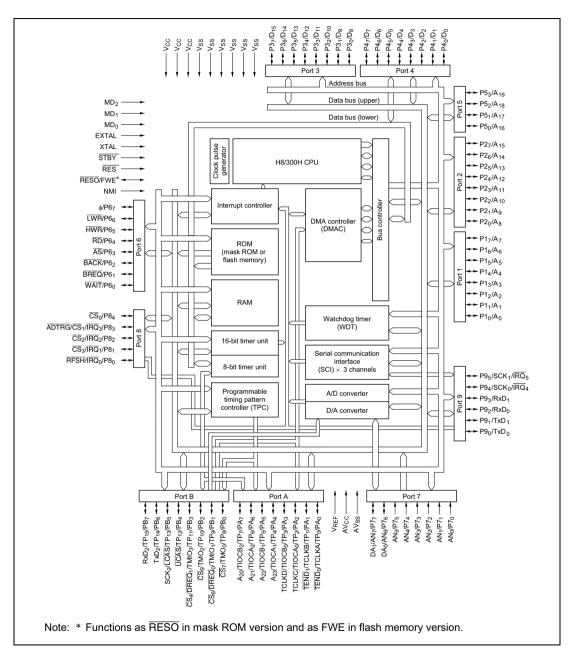
Figure 1.1 Block Diagram
