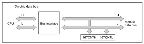
Figure 9.4 16TCNT Access Operation [CPU → 16TCNT (Word)]
