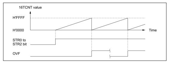
Figure 9.13 Free-Running Counter Operation
