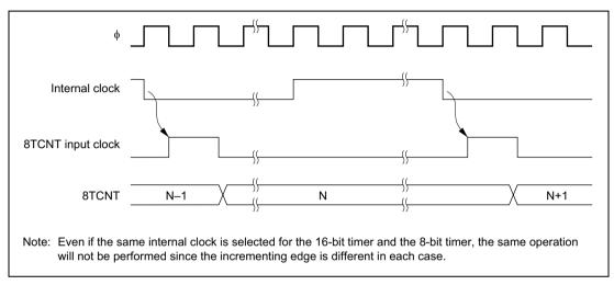
Figure 10.8 Count Timing for Internal Clock Input
