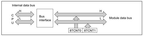
Figure 10.3 8TCNT Access Operation (CPU Reads 8TCNT, Word)
