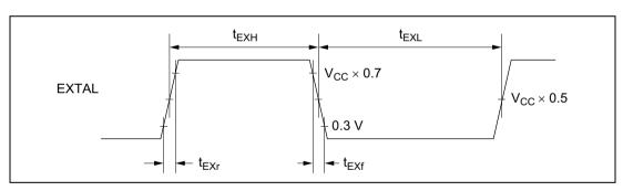
Figure 19.6 External Clock Input Timing
