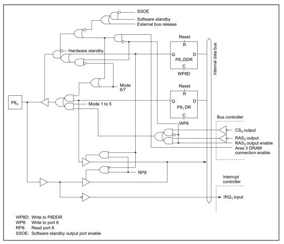
Figure C.8 (b) Port 8 Block Diagram (Pin P81)
