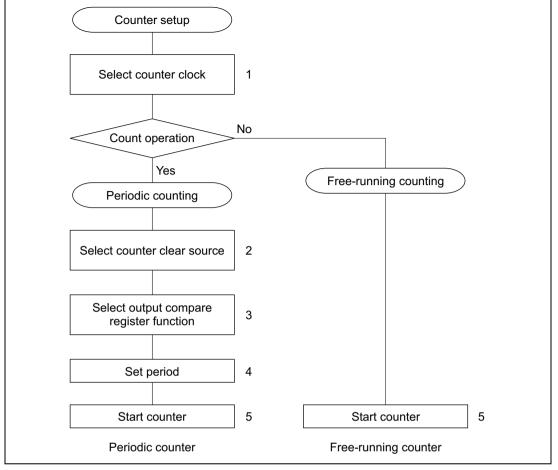
Figure 9.12 Counter Setup Procedure (Example)
