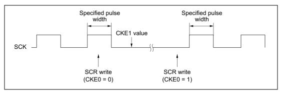
Figure 14.9 Timing for Fixing Cock Output
