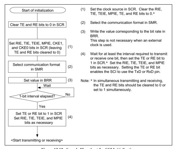
Figure 13.15 Sample Flowchart for SCI Initialization
