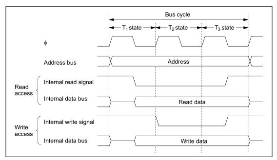
Figure 2.17 Access Cycle for On-Chip Supporting Modules
