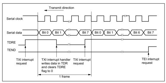
Figure 13.17 Example of SCI Transmit Operation
