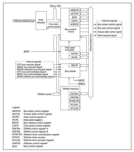
Figure 6.1 Block Diagram of Bus Controller
