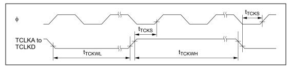
Figure 21.22 Timer External Clock Input Timing
