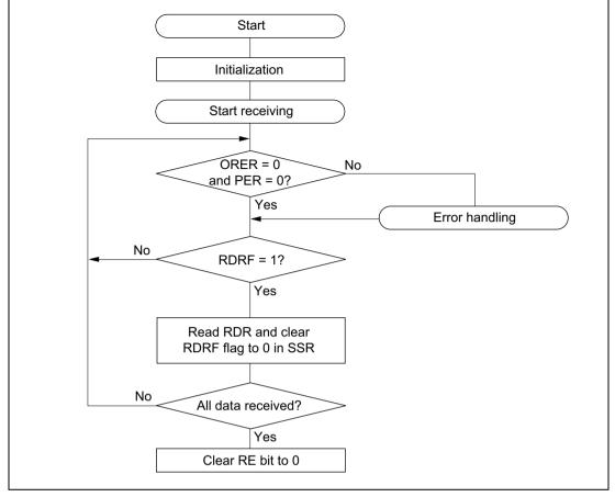
Figure 14.8 Sample Reception Processing Flowchart
