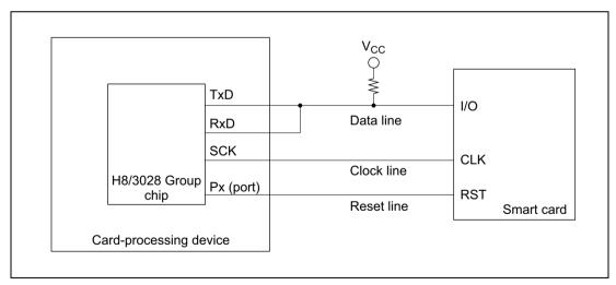
Figure 14.2 Smart Card Interface Connection Diagram
