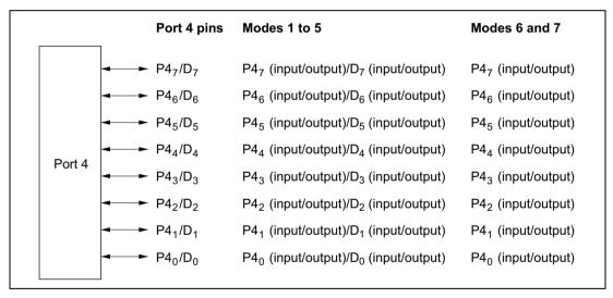
Figure 8.4 Port 4 Pin Configuration
