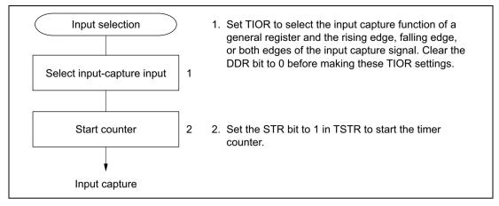
Figure 9.21 Setup Procedure for Input Capture (Example)
