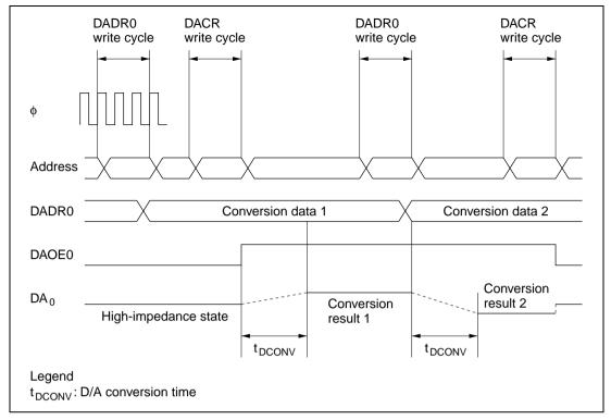
Figure 16.2 Example of D/A Converter Operation
