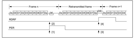
Figure 14.12 Retransmission in SCI Receive Mode
