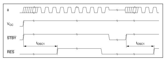
Figure 21.7 Oscillator Settling Timing
