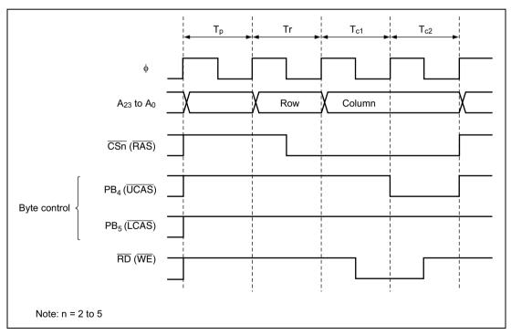
Figure 6.21 Control Timing (Upper-Byte Write Access When CSEL = 0)
