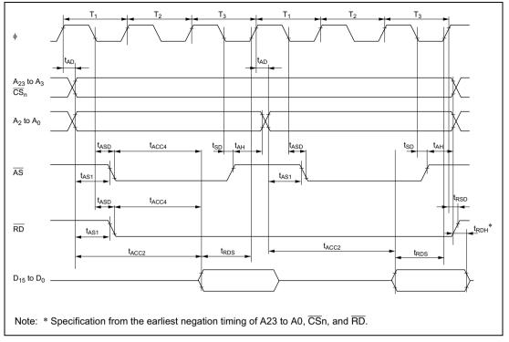
Figure 21.15 Burst ROM Access Timing: Three-State Access
