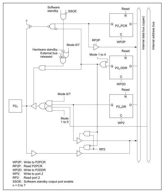
Figure C.2 Port 2 Block Diagram
