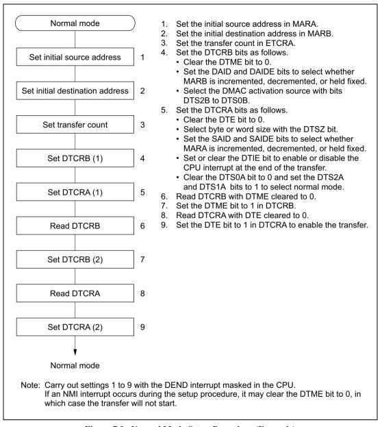
Figure 7.9 Normal Mode Setup Procedure (Example)
