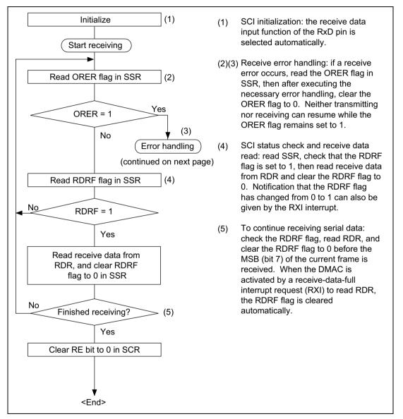
Figure 13.18 Sample Flowchart for Serial Receiving (1)
