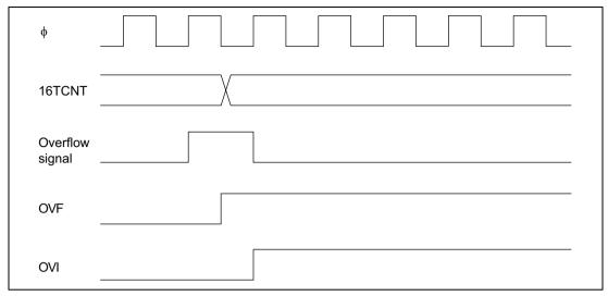
Figure 9.35 Timing of Setting of OVF
