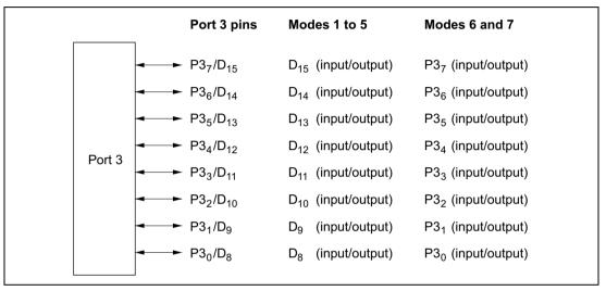
Figure 8.3 Port 3 Pin Configuration
