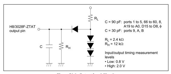
Figure 21.6 Output Load Circuit
