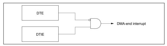
Figure 7.25 DMA-End Interrupt Logic
