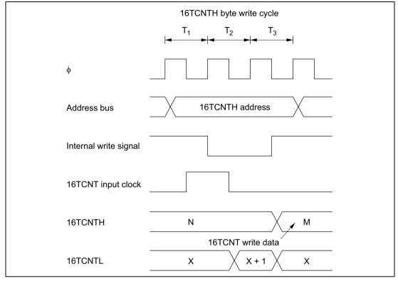
Figure 9.39 Contention between 16TCNT Byte Write and Increment
