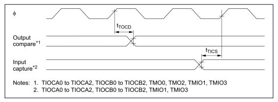
Figure 21.21 Timer Input/Output Timing
