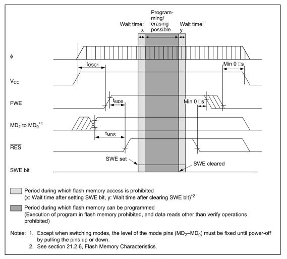
Figure 18.16 Power-On/Off Timing (Boot Mode)
