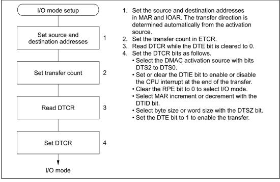
Figure 7.3 I/O Mode Setup Procedure (Example)
