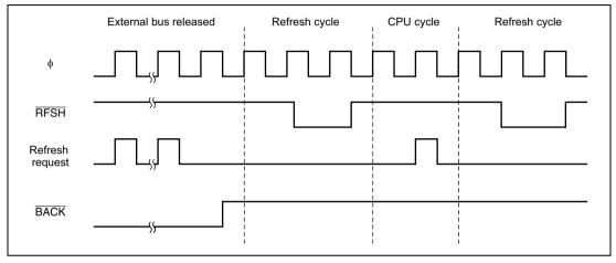
Figure 6.35 Bus-Released State and Refresh Cycles
