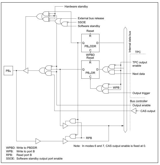
Figure C.11 (e) Port B Block Diagram (Pin PB<sub>4</sub>)
