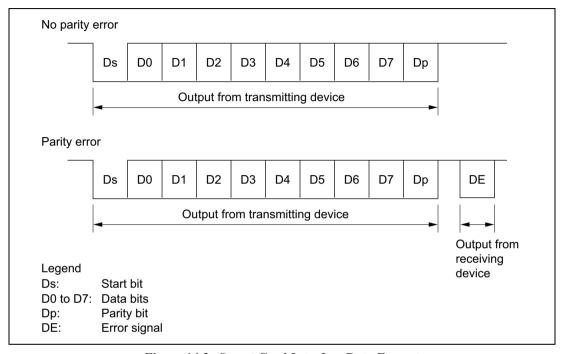
Figure 14.3 Smart Card Interface Data Format
