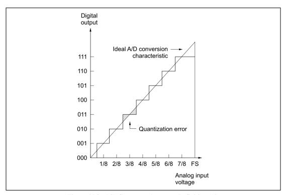
Figure 15.9 A/D Converter Accuracy Definitions (1)
