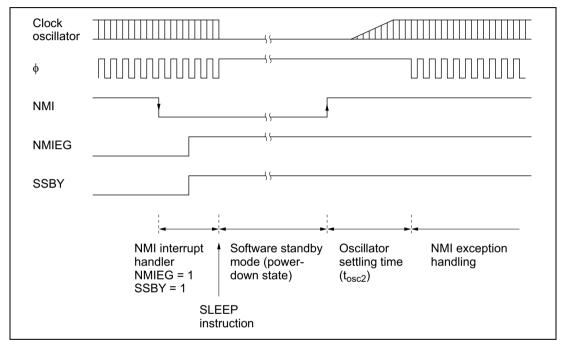
Figure 20.1 NMI Timing for Software Standby Mode (Example)
