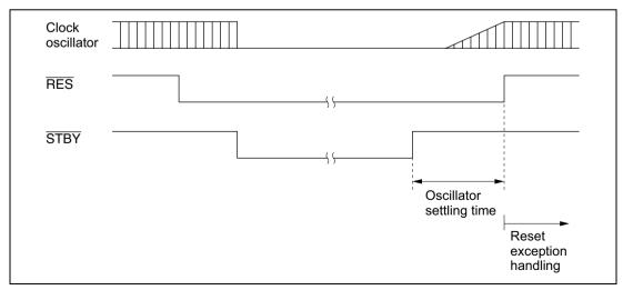
Figure 20.2 Hardware Standby Mode Timing
