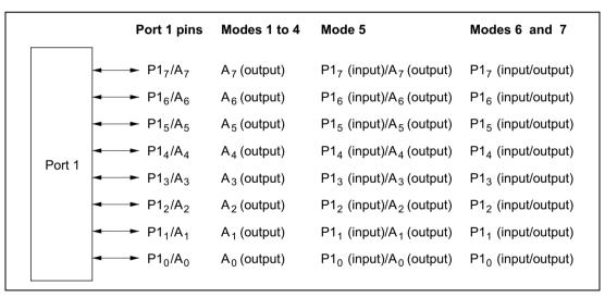
Figure 8.1 Port 1 Pin Configuration
