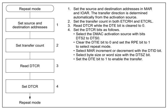
Figure 7.7 Repeat Mode Setup Procedure (Example)
