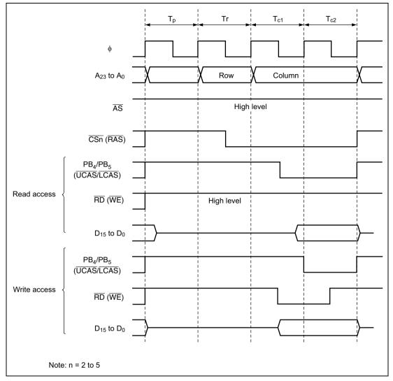
Figure 6.18 Basic Access Timing (CSEL = 0 in DRCRB)
