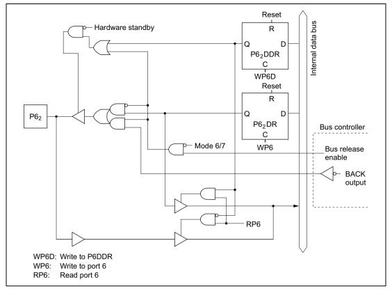
Figure C.6 (c) Port 6 Block Diagram (Pin P62)
