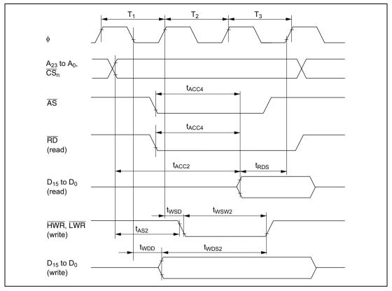
Figure 21.12 Basic Bus Cycle: Three-State Access
