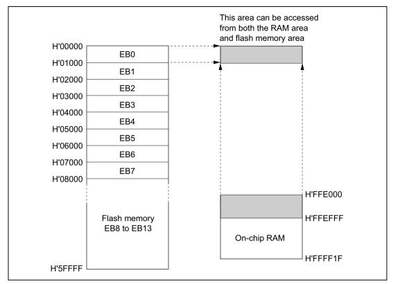
Figure 18.14 Example of RAM Overlap Operation
