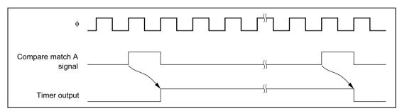
Figure 10.10 Timing of Timer Output
