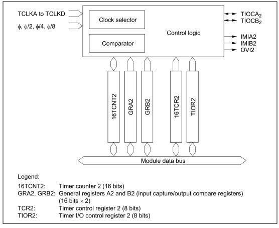
Figure 9.3 Block Diagram of Channel 2
