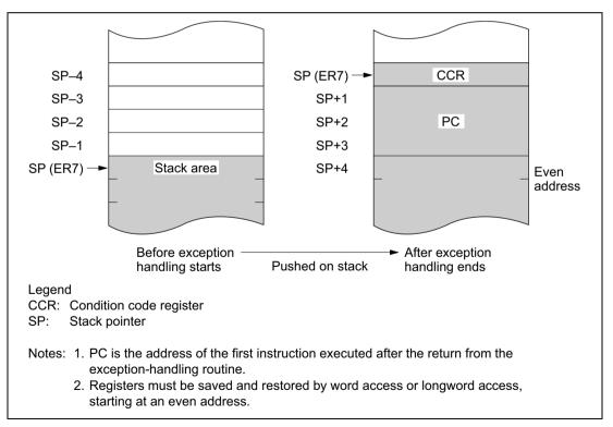
Figure 2.14 Stack Structure after Exception Handling
