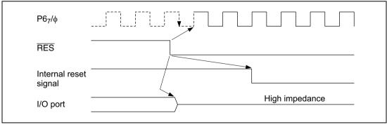
Figure D.4 Reset during Operation (Modes 6 and 7)
