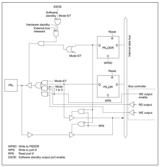
Figure C.6 (e) Port 6 Block Diagram (Pin P64)
