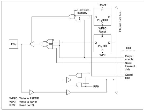
Figure C.9 (a) Port 9 Block Diagram (Pin P9<sub>0</sub>)
