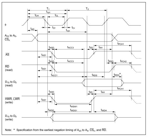
Figure 21.11 Basic Bus Cycle: Two-State Access
