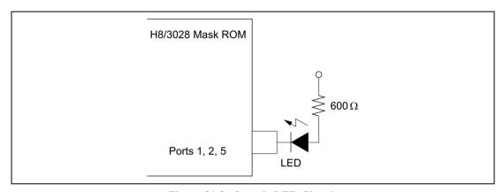
Figure 21.2 Sample LED Circuit
