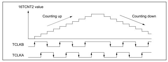
Figure 9.30 Operation in Phase Counting Mode (Example)
