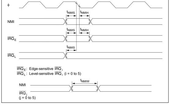
Figure 21.10 Interrupt Input Timing
