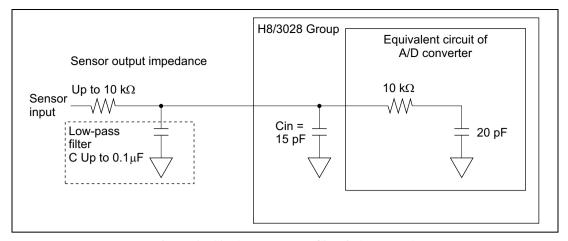
Figure 15.11 Analog Input Circuit (Example)
