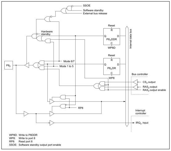
Figure C.8 (c) Port 8 Block Diagram (Pin P82)
