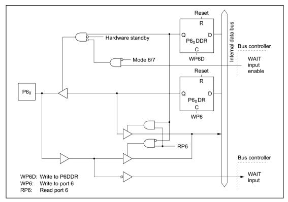
Figure C.6 (a) Port 6 Block Diagram (Pin P6<sub>0</sub>)
