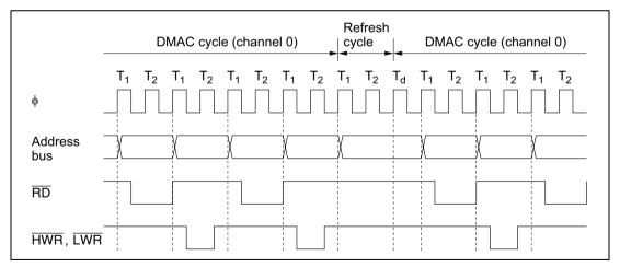
Figure 7.20 Bus Timing of DRAM Interface, and DMAC
