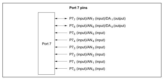
Figure 8.7 Port 7 Pin Configuration
