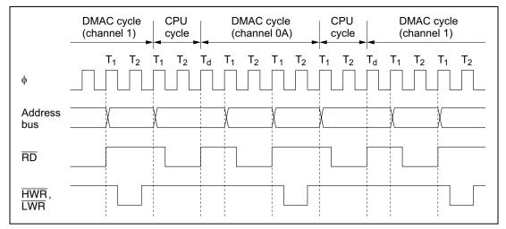
Figure 7.19 Timing of Multiple-Channel Operations
