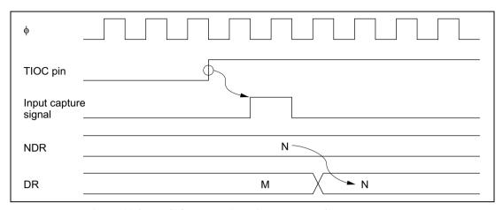
Figure 11.8 TPC Output Triggering by Input Capture (Example)
