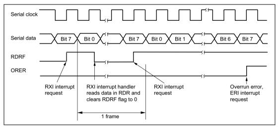
Figure 13.19 Example of SCI Receive Operation
