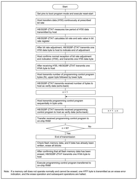
Figure 18.6 Boot Mode Execution Procedure
