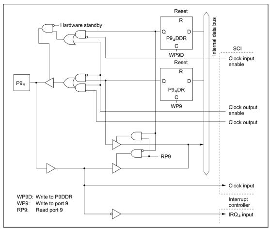
Figure C.9 (e) Port 9 Block Diagram (Pin P9<sub>4</sub>)
