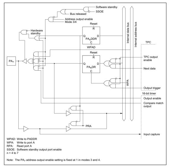
Figure C.10 (c) Port A Block Diagram (Pins PA<sub>4</sub> to PA<sub>7</sub>)
