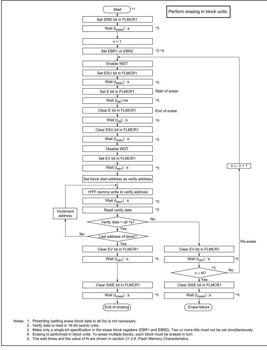
Figure 18.11 Erase/Erase-Verify Flowchart (Single-Block Erasing)
