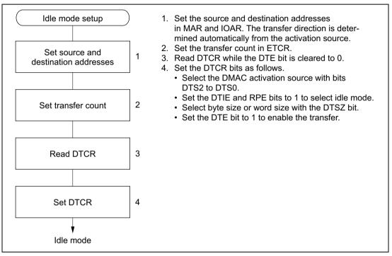
Figure 7.5 Idle Mode Setup Procedure (Example)
