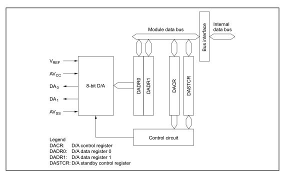
Figure 16.1 D/A Converter Block Diagram
