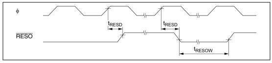
Figure 21.9 Reset Output Timing\*
