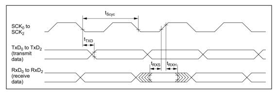
Figure 21.24 SCI Input/Output Timing in Synchronous Mode
