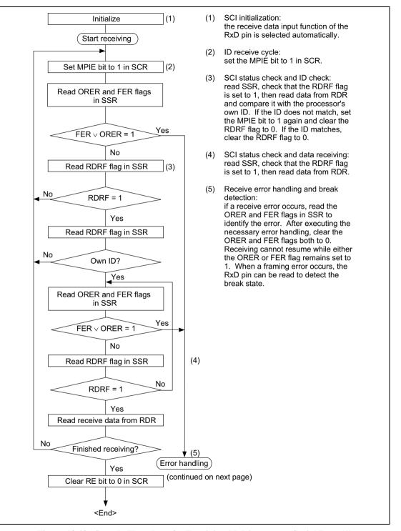
Figure 13.12 Sample Flowchart for Receiving Multiprocessor Serial Data (1)
