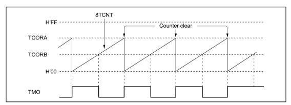
Figure 10.17 Example of Pulse Output
