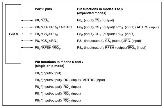
Figure 8.8 Port 8 Pin Configuration
