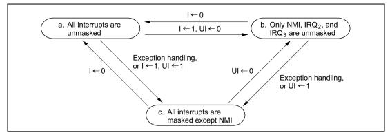
Figure 5.5 Interrupt Masking State Transitions (Example)
