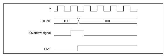
Figure 10.16 Timing of OVF Setting
