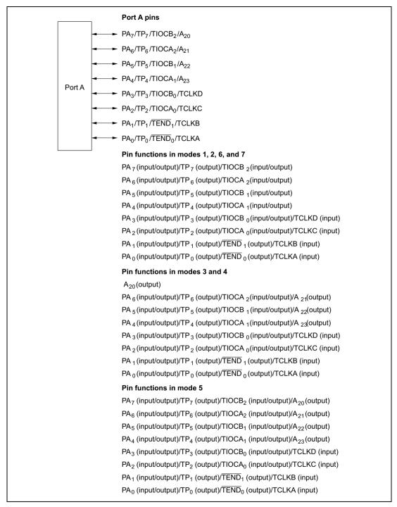
Figure 8.10 Port A Pin Configuration
