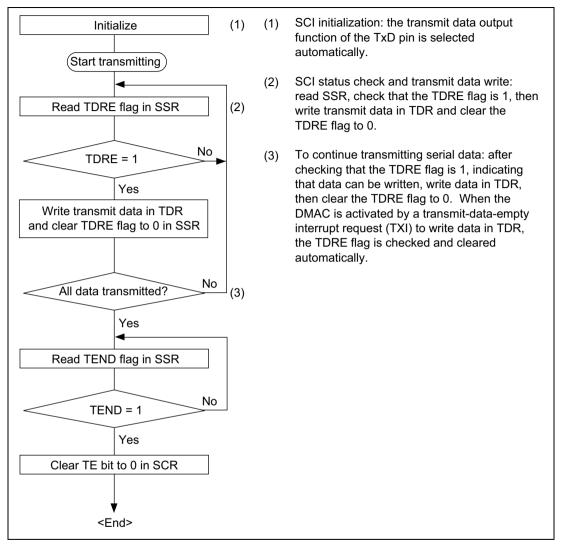
Figure 13.16 Sample Flowchart for Serial Transmitting
