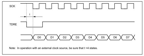
Figure 13.22 Example of Synchronous Transmission Using DMAC
