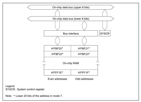
Figure 17.1 RAM Block Diagram
