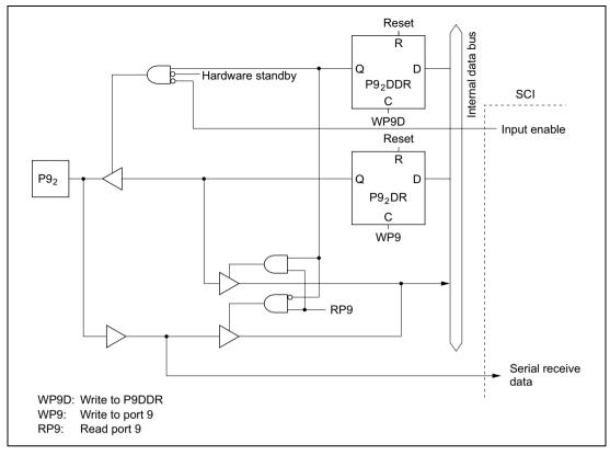
Figure C.9 (c) Port 9 Block Diagram (Pin P92)
