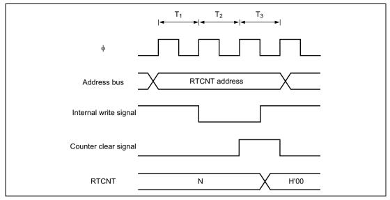
Figure 6.39 Contention between RTCNT Write and Clear
