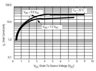
Figure 3. Typical LED Output I-V Characteristic
