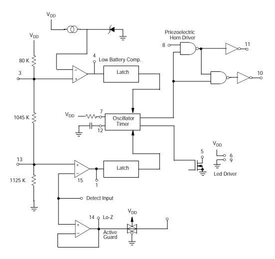
Figure 2. Block Diagram
