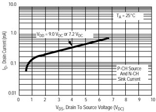
Figure 4. Typical Comparator Output I-V Characteristic
