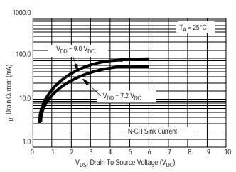
Figure 5. Typical P Horn Driver Output I-V Characteristic
