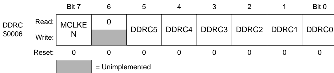
Figure 8. Data direction register C (DDRC)
