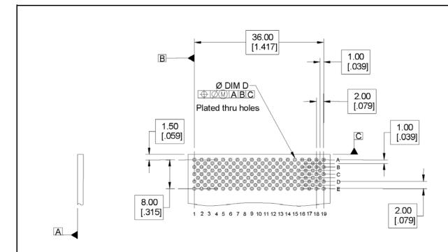
Recommended PCB hole mounting pattern for coaxial, column diferential and stripline applications
