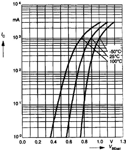
**Collector current  $I_C = f(V_{BE})$**
