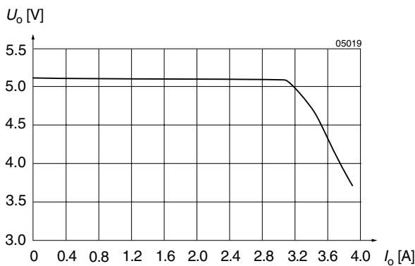
Fig. 11 U_o versus I_o (typ) of units with U_o = 5.1 V. (110 IMY 15-05-7R)
