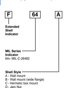
E - Hermetic jam nut F - Straight plug Shell Size
