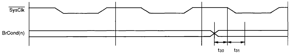
Figure 21. Direct Branch Condition Input Timing
