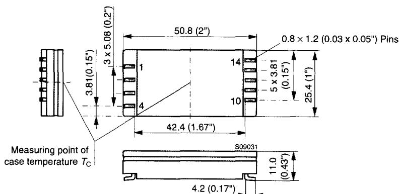
**IML SMD version (option L)**
