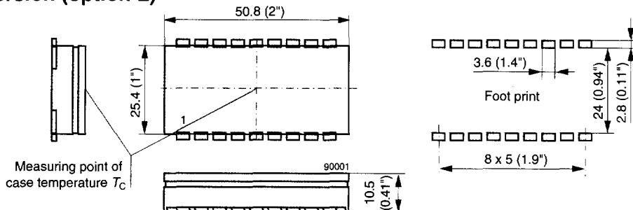
**Pin allocation IML, option M and Z**
