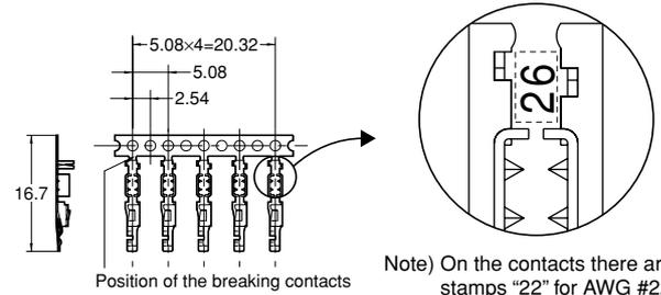
Note) On the contacts there are stamps "22" for AWG #22 and #24 types, and "26" for AWG #26 and #28 types.
