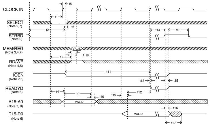
FIGURE 16. CPU READING RAM (SHOWN FOR 16-BIT, BUFFERED, NONZERO WAIT MODE, UNCONTENDED ACCESS)
