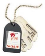
The P-tag connector will be implemented in Readers and Host Devices. It will also be used in a multitude of Host Devices for the Military and Medical Industry. It has ten contacts in 2.00mm pitch and two grounding pads with unshielded top-mount type. The P-Tag Connector is 33.5mm length, 37.07mm width and 4.32mm thickness.
