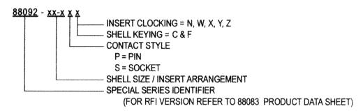
Plug Connector, Arctic Coupling Ring, Bayonet Coupling
