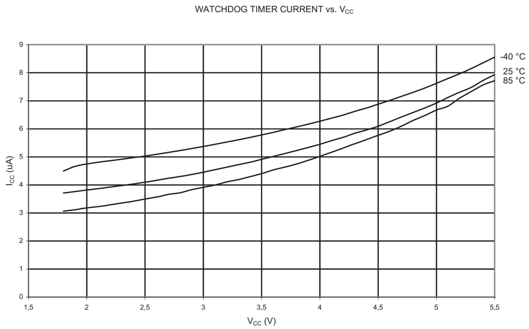
Figure 17-50. Watchdog Timer Current vs. V_{CC}
