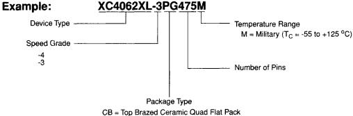
CB = Top Brazed Ceramic Quad Fla PG = Ceramic Pin Grid Array
