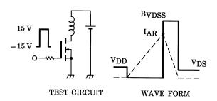
$$\begin{aligned} &RG = 25 \ \Omega \\ &V_{DD} = 50 \ V, \ L = 1.2 \ mH \end{aligned} \qquad EAS = \frac{1}{2} \cdot L \cdot I^2 \cdot \left( \frac{BVDSS}{BVDSS - VDD} \right)$$
