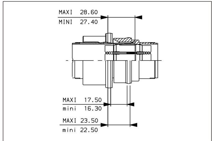
During the mating operation, the receptacle comes up to plug. The front of plug enters in receptacle cone. When plug touches the cone, this induces a lateral movement of plug shell relatively to the flange fixed on panel. This movement stops when the plug shell axis is in conformance with the receptacle ones.
