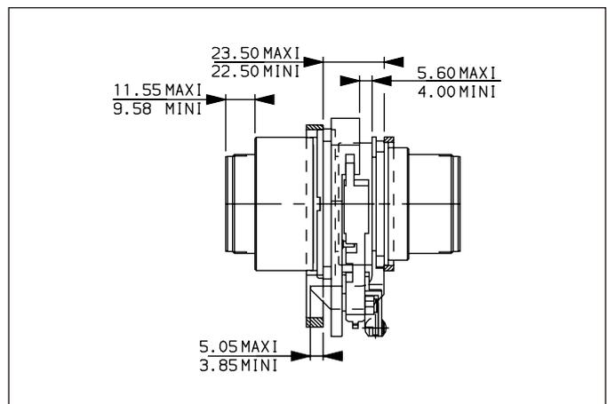
The Launching Security Device is designed to catch the floating connector plug shell during the flight.
