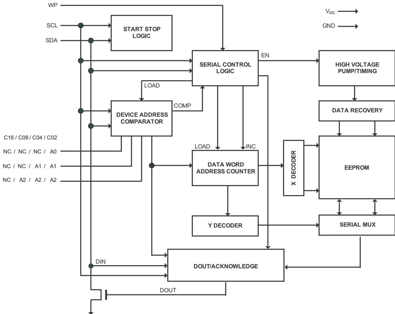
Figure 1. Block Diagram
