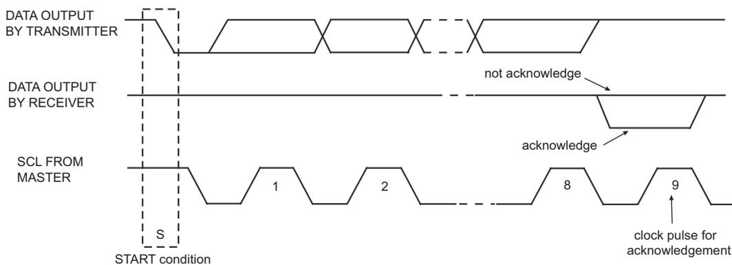
Figure 7. Acknowledge on the I<sup>2</sup>C bus
