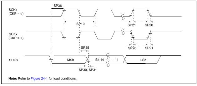
TABLE 24-33: SPIX MASTER MODE (HALF-DUPLEX, TRANSMIT ONLY) TIMING REQUIREMENTS
