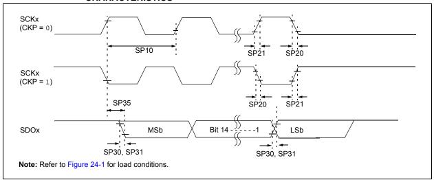
FIGURE 24-15: SPIX MASTER MODE (HALF-DUPLEX, TRANSMIT ONLY CKE = 1) TIMING CHARACTERISTICS
