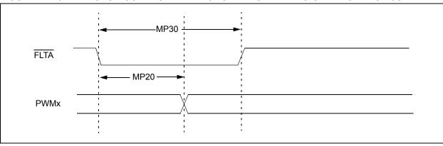
FIGURE 24-11: MOTOR CONTROL PWM MODULE TIMING CHARACTERISTICS
