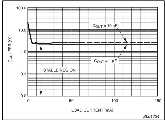
Figure 14. Region of stable C<sub>OUT</sub> ESR versus load current.
