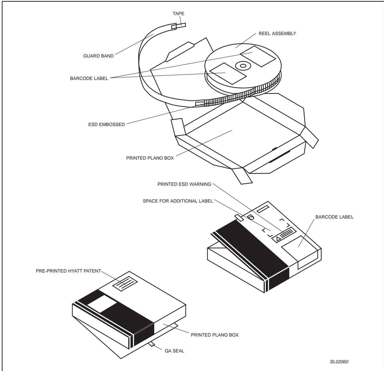
Figure 23. WL-CSP5 tape and reel packing method.
