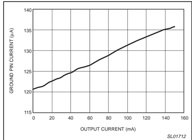
Figure 4. GND pin current versus output current.
