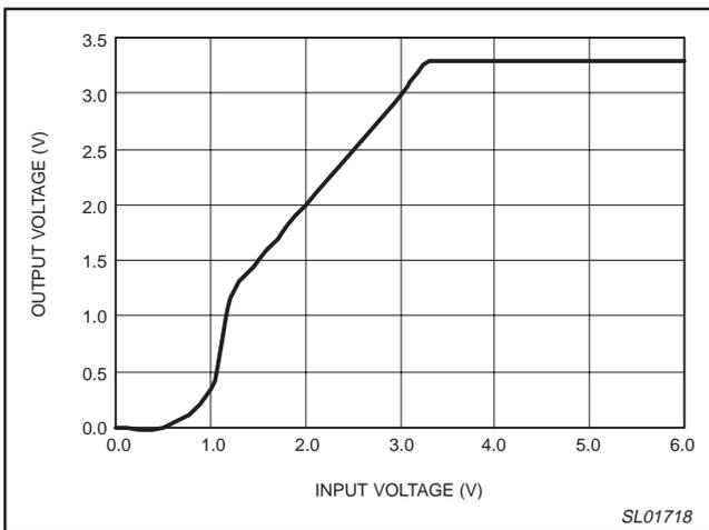
Figure 11. Output voltage (no load) versus input voltage.
