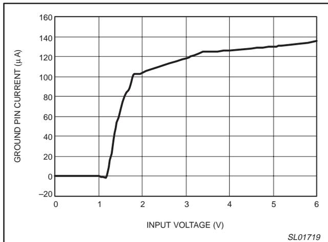
Figure 7. GND pin current (50 mA) versus input voltage.
