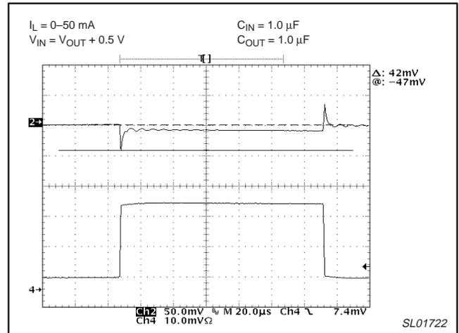
Figure 19. Load transient response (with AA battery source).
