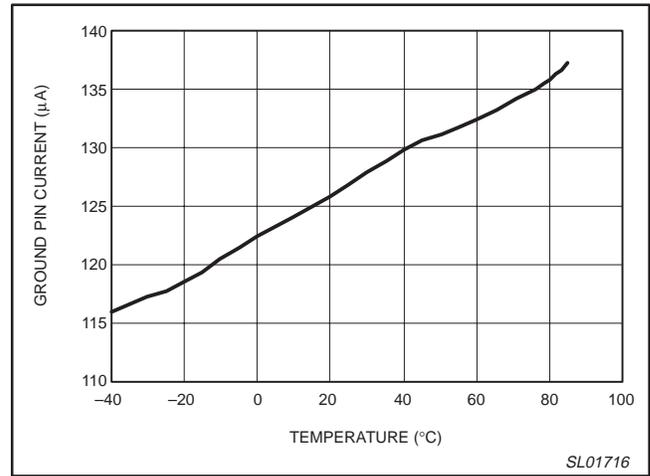
Figure 10. GND pin current (50 mA load) versus temperature.
