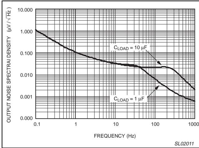
Figure 13. Output noise spectral density versus frequency.
