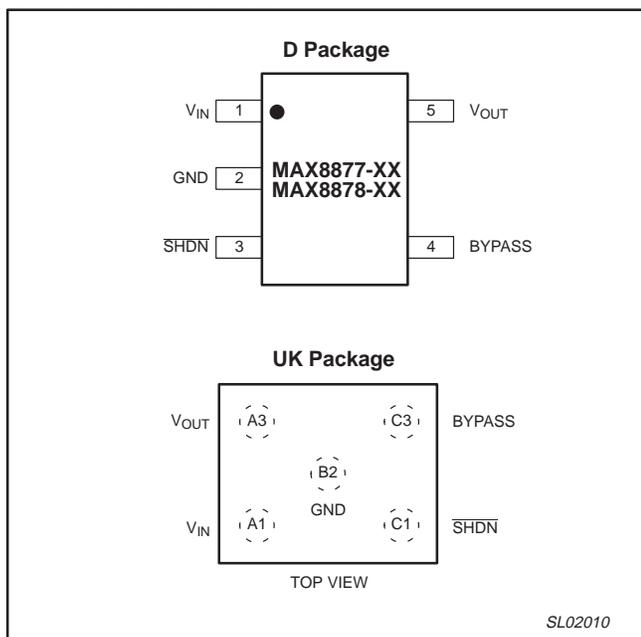
Figure 2. Pin configurations.
