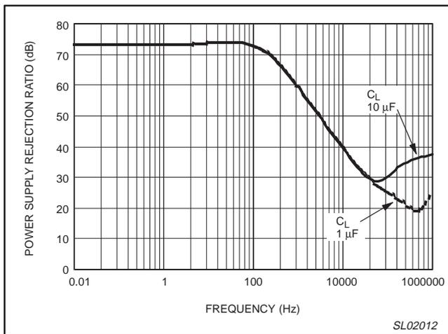
Figure 15. Power supply rejection ratio versus frequency.
