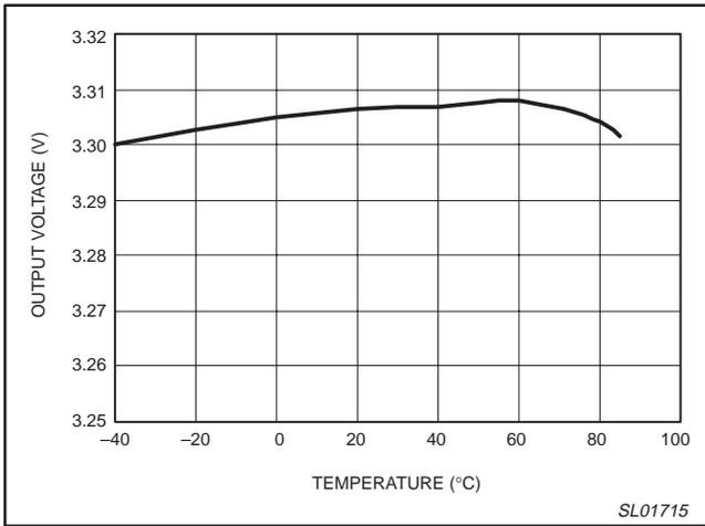
Figure 9. Output voltage (50 mA load) versus temperature.
