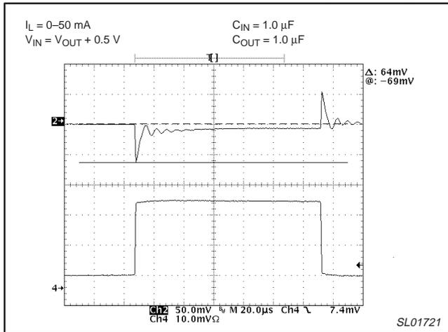
Figure 18. Load transient response (with power supply source).
