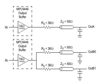
Figure 3. Single versus Dual Transmission Lines
