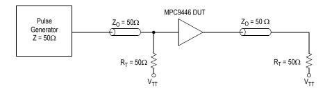
Figure 6. CCLK0, 1 MPC9446 AC Test Reference for V<sub>CC</sub> = 3.3 V and V<sub>CC</sub> = 2.5 V
