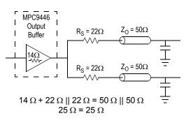
Figure 5. Optimized Dual Line Termination
