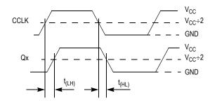
Figure 8. Propagation Delay (t<sub>PD</sub>) Test Reference
