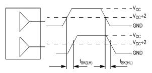
The pin-to-pin skew is defined as the worst case difference in propagation delay between any two similar delay paths within a single device.
