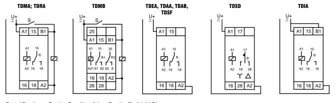
Control Function Function Rp: without link Function Ri: link A1-B1
