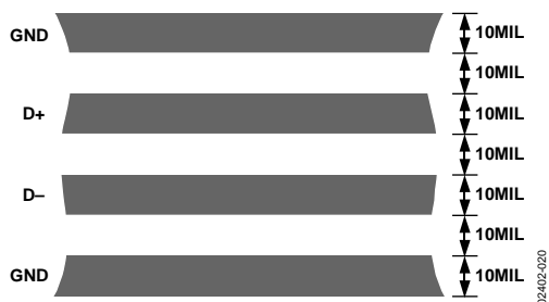
Figure 20. Arrangement of Signal Tracks
