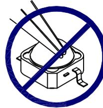
3. Do not stack together assembled PCBs containing exposed LEDs. Impact may scratch the silicone lens or damage the internal circuitry.
