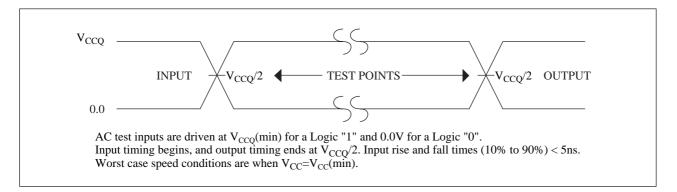
Figure 4. Transient Input/Output Reference Waveform for  $V_{CC}$ =2.7V-3.3V
