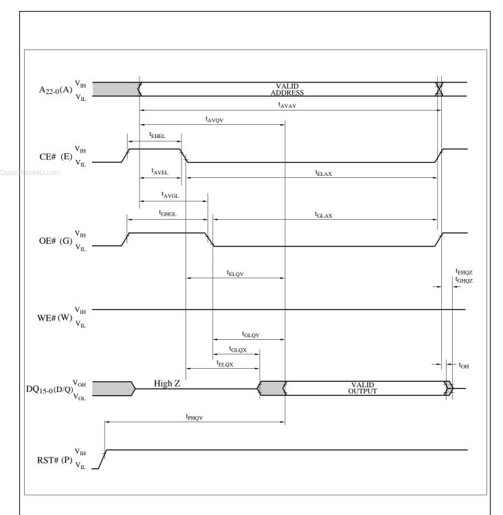
Figure 6. AC Waveform for Single Asynchronous Read Operations from Status Register, Identifier Codes, OTP Block or Query Code
