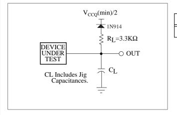
Figure 5. Transient Equivalent Testing Load Circuit
