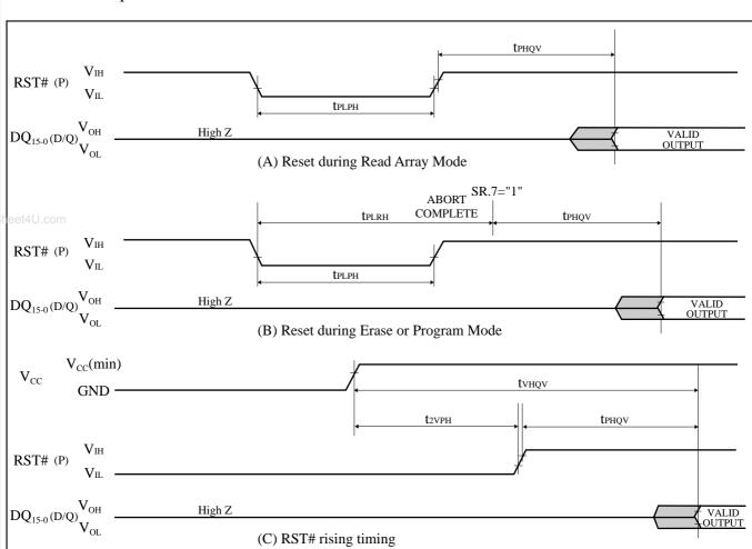
Figure 10. AC Waveform for Reset Operations
