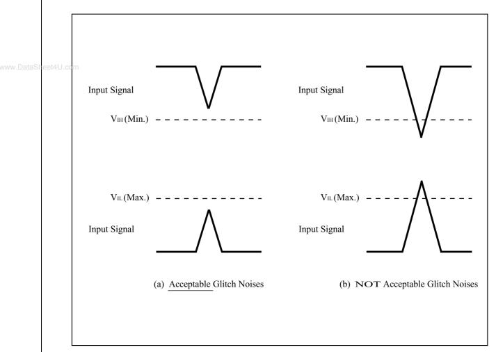
Figure A-2. Waveform for Glitch Noises
