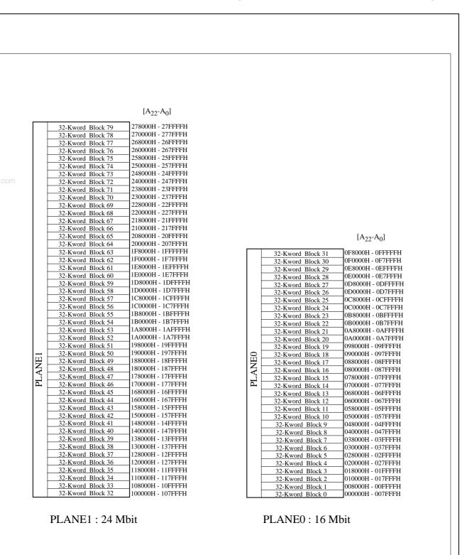
Figure 2.1. Memory Map (Top Parameter, Plane 0 and Plane 1)
