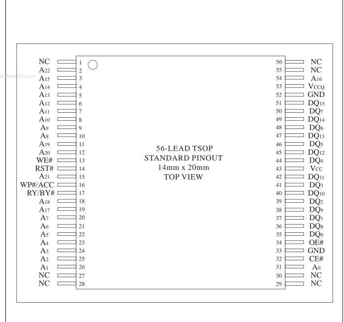
Figure 1. 56-Lead TSOP (Normal Bend) Pinout
