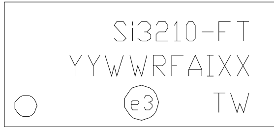
Figure 40. TSSOP Top Mark Diagram
