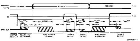
Switching delays from address and chip select inputs to the data output. For the Am93425SA/A/425, disabled output is OFF, represented by a single center line. For the Am93415SA/A/415, a disabled output is HIGH.
