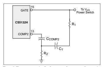
Figure 7: Slope compensation for the non-synchronous regulator section ( $V_{\mathrm{I/O}}$ ).
