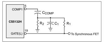
Figure 6: Small RC filter provides the proper voltage ramp at the begining of each on-time cycle.
