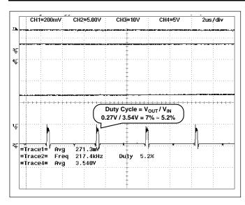
Figure 4: Pulse-by-Pulse Regulation during Soft Start (2µs/div).
