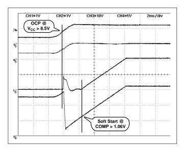
Figure 5: Start-up with COMP pre-charged to 2V (2ms/div).
