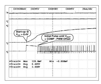
Figure 3: Normal Start-up showing initial pulse followed by Soft Start (20μs/div).
