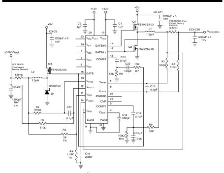
5V/12V to 2V/16A for Pentium  $^{\circledast}$  II  $V_{CC(CORE)}$  , 5V/12V to 3.3V/8A for  $V_{I/O}$
