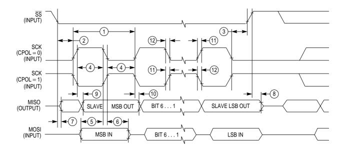
Figure A-8 SPI Slave Timing (CPHA =1)
