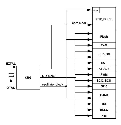
**Figure 3-1 Clock Connections**
