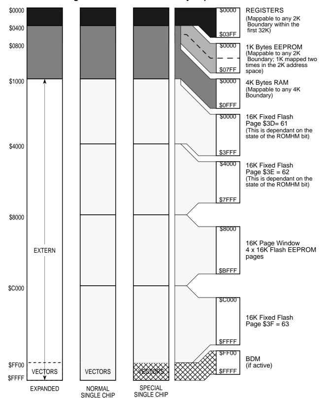
Figure 1-2 MC9S12DJ64 Memory Map out of Reset
