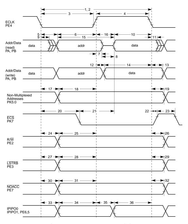
Figure A-9 General External Bus Timing
