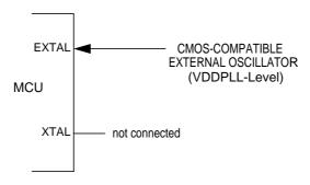
Figure 2-6 External Clock Connections (PE7=0)
