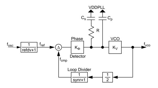
Figure A-2 Basic PLL functional diagram
