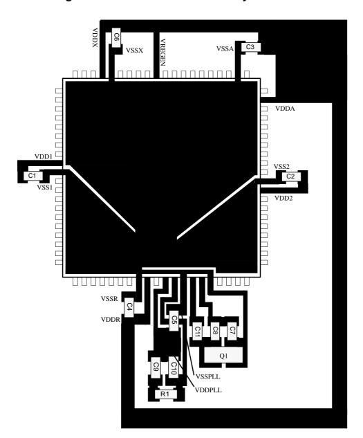
Figure 20-2 Recommended PCB Layout for 80QFP
