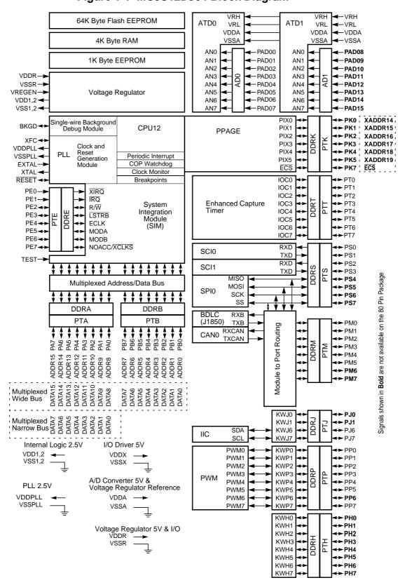
Figure 1-1 MC9S12DJ64 Block Diagram
