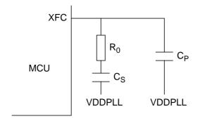
Figure 2-3 PLL Loop Filter Connections
