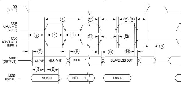
Figure A-7 SPI Slave Timing (CPHA = 0)
